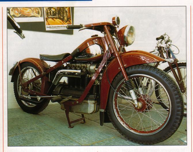
ABOVE: A telescopic-forked 1955 Nimbus overhead camshaft, four-cylinder machine of 746cc (45.50cu. in.) displacement. It used a pressed steel frame. Despite upgrades, Nimbus products remained very similar over 37 years.
