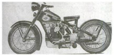
Altho the "Nimbus" has telescopic front forks, the rear wheel is mounted rigid. Frame is of flat strap metal construction. Shaft drive is employed.
