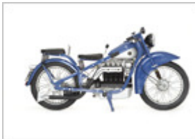
Nimbus, Four, 1946 , Denmark, 746 cc, 22hp, SOHC.
