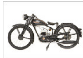
Husqvarna "mod.24", Single, 1949 , Sweden, 118cc, 3 1/2hp, Two Stroke.
