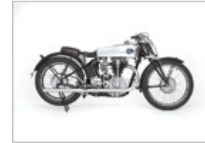
NSU 500 SS Racer, Single 1932, Germany, 494 cc, 20hp, SOHC.
