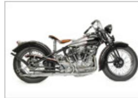
Crocker "Big Tank", V-Twin, 1939 , United States, 1000 cc, 60hp, OVH.
