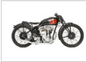
Excelsior Manxman, Racer, Single, 1935 , England, 246 cc, hp unknown, SOHC.
